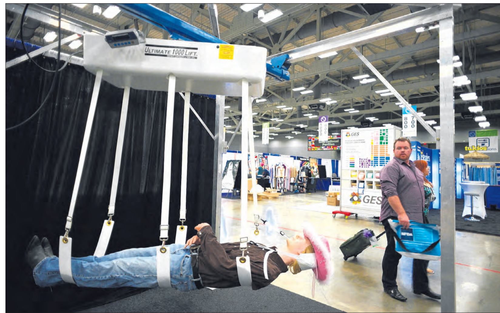
A body lift fitted with a sling holding a cowboy mannequin at the Mortuary Lift Company booth. The body lift, which is used in mortuaries and funeral homes, makes lighter work of lifting and moving bodies and caskets around. It also comes in handy during the dressing process.
